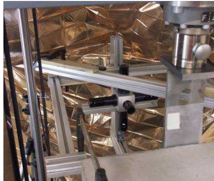
Fig. 4.1: Stiff connection between interferometer and concrete, shading to reduce outer light
