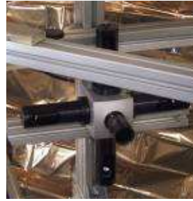
Fig. 3.2: Speckle interferometer with 4 reflector arms
